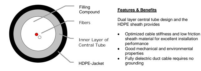
Principle drawing for an A-D2Y 1x2 E9XB/125 0,36F3,5 + 0,22H18
